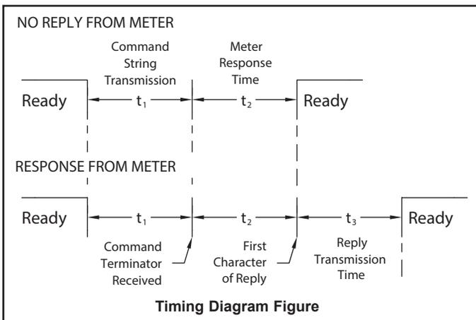
At the start of the time interval  $t_1$ , the computer program prints or writes the string to the com port, thus initiating a transmission. During  $t_1$ , the command characters are under transmission and at the end of this period, the command terminating character (\*) is received by the meter. The time duration of  $t_1$  is dependent on the number of characters and baud rate of the channel.
