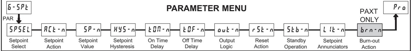
▽ - A setpoint card must be installed in order to access this module.
