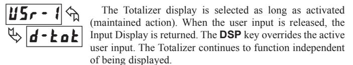
The Totalizer display is selected as long as activated (maintained action). When the user input is released, the Input Display is returned. The **DSP** key overrides the active user input. The Totalizer continues to function independent of being displayed.
