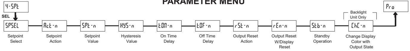
The Setpoint Output Parameters are only active when an optional output module is installed in the meter.
