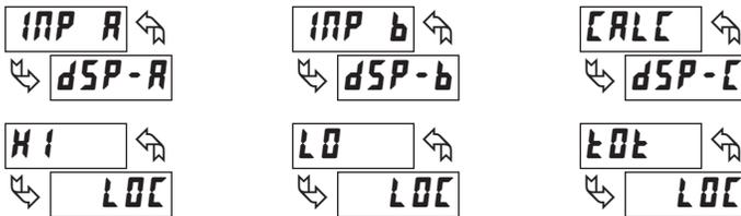
There are six meter values that can be individually programmed for one of the main displays (A,B,C or \_), or programmed to be viewable in Quick Programming mode (**rEd**), or programmed to be locked out from display (**LOC**) (see the following table). If two or more values are assigned to the same display the last value assigned will be the one that is displayed.
