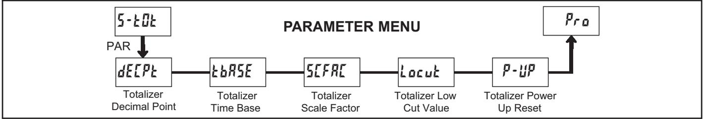
The totalizer accumulates (integrates) the Input Display value using one of two modes. The first is using a time base. This can be used to compute a time-temperature product. The second is through a user input or function key programmed for Batch (one time add on demand). This can be used to provide a readout of temperature integration, useful in curing and sterilization applications. If the Totalizer is not needed, its display can be locked-out and this module can be skipped during programming.
