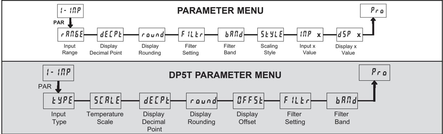
Refer to the appropriate Input Range for the selected meter. Use only one Input Range, then proceed to Display Decimal Point.
