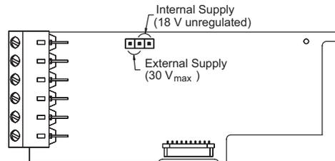
2. Install the plug-in card by aligning the card terminals with the slot bay in the rear cover. Be sure the connector is fully engaged and the tab on the plug-in card rests in the alignment slot on the display board.
