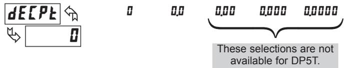
Select the decimal point location for the Input, MAX and MIN displays. (The TOT display decimal point is a separate parameter.) This selection also affects round, dSP 1 and dSP 2 parameters.
