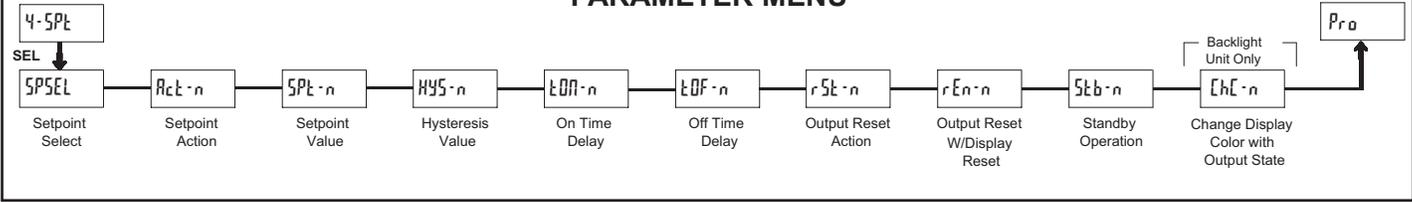
The Setpoint Output Parameters are only active when an optional output module is installed in the meter.
