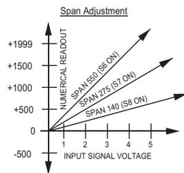
The approximate span contributed by each switch is shown on the rear label. The values shown are "units per volt." For example, if S6 only is turned "ON," the numerical readout will change approximately 550 units for a signal voltage change of 1 volt. If S7 were also turned "ON," the numerical readout would change approximately 825 units for a signal voltage change of 1 volt. The span adjust pot has a continuous span range of approximately 0- 45.
