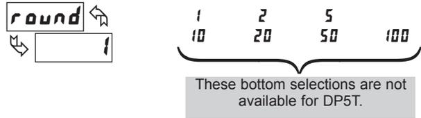
Rounding selections other than one, cause the Input Display to 'round' to the nearest rounding increment selected (ie. rounding of '5' causes 122 to round to 120 and 123 to round to 125). Rounding starts at the least significant digit of the Input Display. Remaining parameter entries (scaling point values, etc.) are not automatically adjusted to this display rounding selection.
