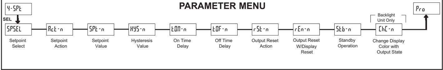
The Setpoint Output Parameters are only active when an optional output module is installed in the meter.
