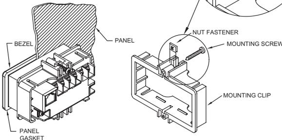
panel latch should be engaged in the farthest forward slot possible. To achieve a proper seal, tighten the latch screws evenly until the unit is snug in the panel (Torque to approx. 28 to 36 in-oz [0.202 to 0.26 N-m]). Do not over-tighten the screws.
