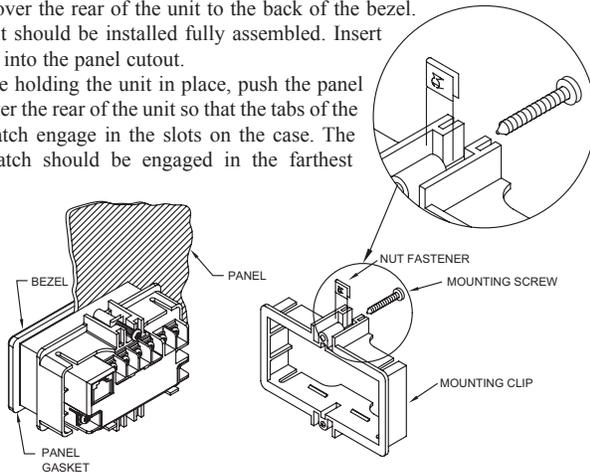
forward slot possible. To achieve a proper seal, tighten the latch screws evenly until the unit is snug in the panel (Torque to approx. 28 to 36 in-oz [0.202 to 0.26 N-m]). Do not over-tighten the screws.
