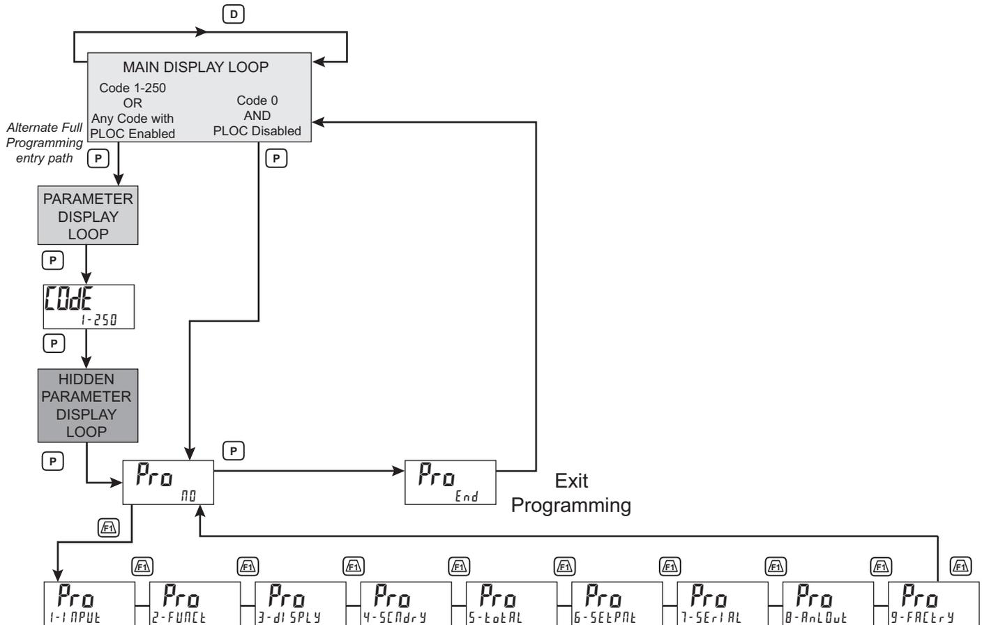
\* Pressing "D" at any time exits back to the Main Display Loop.
