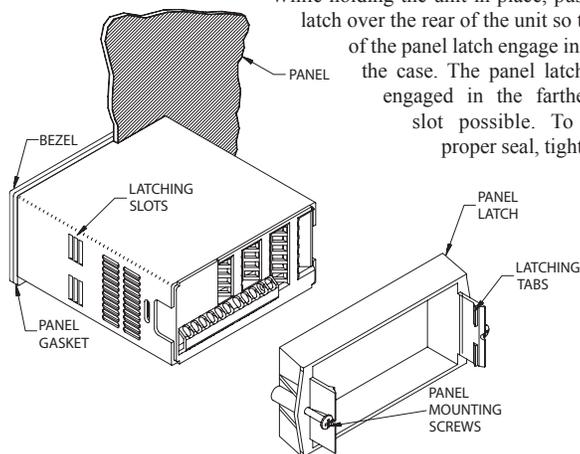
screws evenly until the unit is snug in the panel (Torque to approximately 7 in-lbs [79N-cm]). Do not over-tighten the screws.
