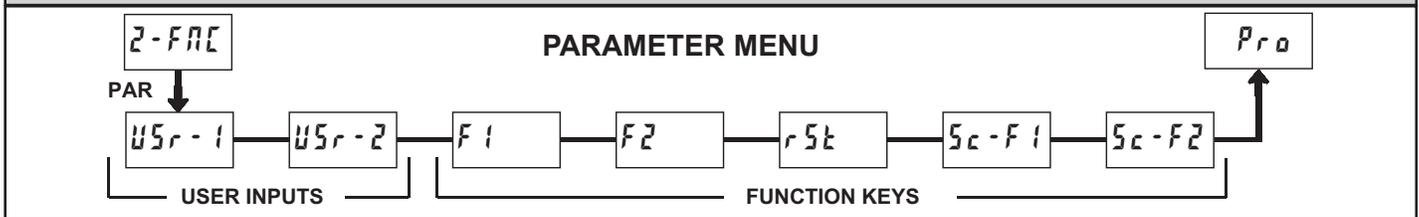
The two user inputs are individually programmable to perform specific meter control functions. While in the Display Mode or Program Mode, the function is executed the instant the user input transitions to the active state.
