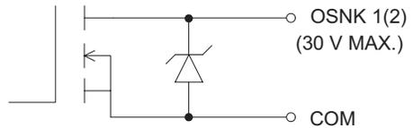
Output Common is not isolated from DC Power Common. Load must be wired between OSNK terminal and V+ of the load supply.
