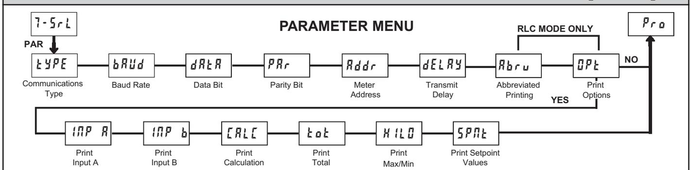
▽ - A communication card must be installed in order to access this module.
