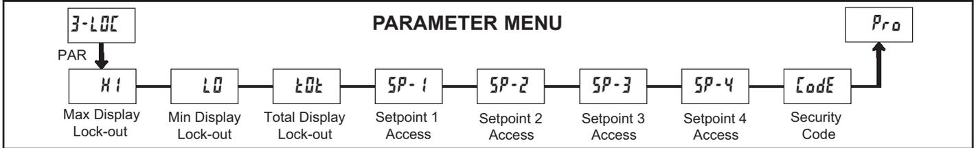
Module 3 is the programming for Display lock-out and “Full” and “Quick” Program lock-out.
