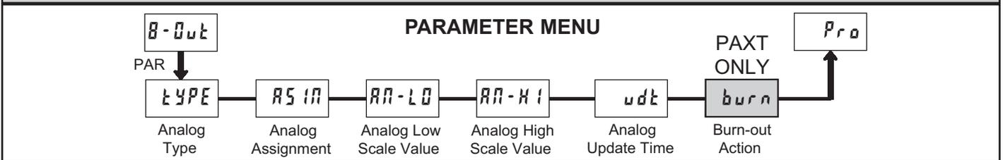
▽ - An analog output card must be installed in order to access this module.
