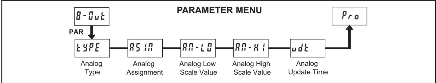
▽ - An analog output card must be installed in order to access this module.
