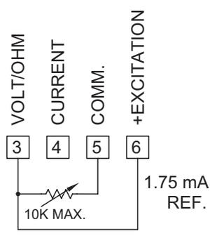
**Potentiometer Signal (3 wire requiring excitation)**
