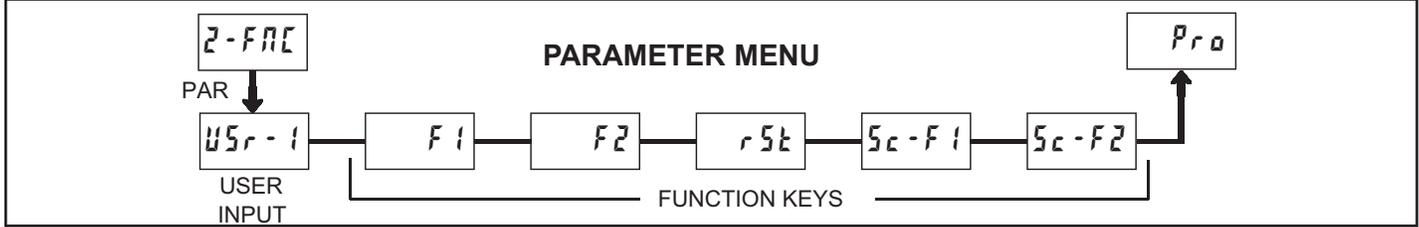
The user input is programmable to perform specific meter control functions. While in the Display Mode or Program Mode, the function is executed the instant the user input transitions to the active state.
