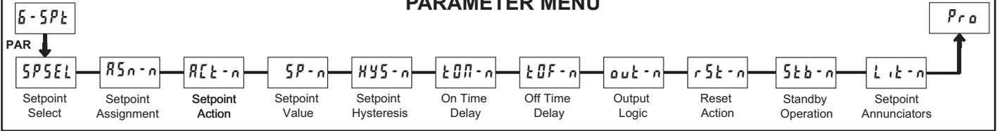
▽ - A setpoint card must be installed in order to access this module.
