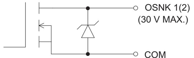
Output Common is not isolated from DC Power Common. Load must be wired between OSNK terminal and V+ of the load supply.
