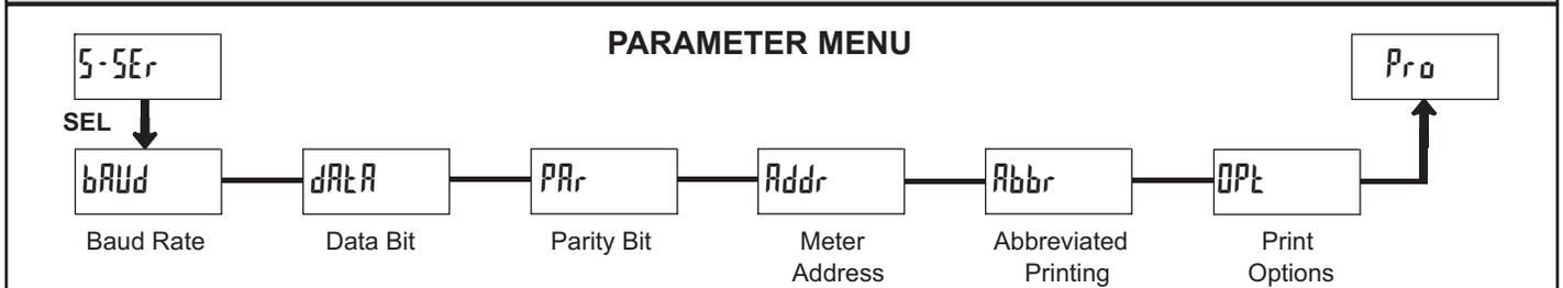
The Serial Setup Parameters are only active when one of the optional serial communication/programming cards is installed in the meter.
