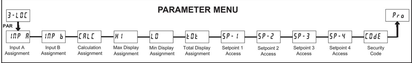
Module 3 is the programming for the Display, Display assignments, Display lock-out and “Full” and “Quick” Program lock-out.
