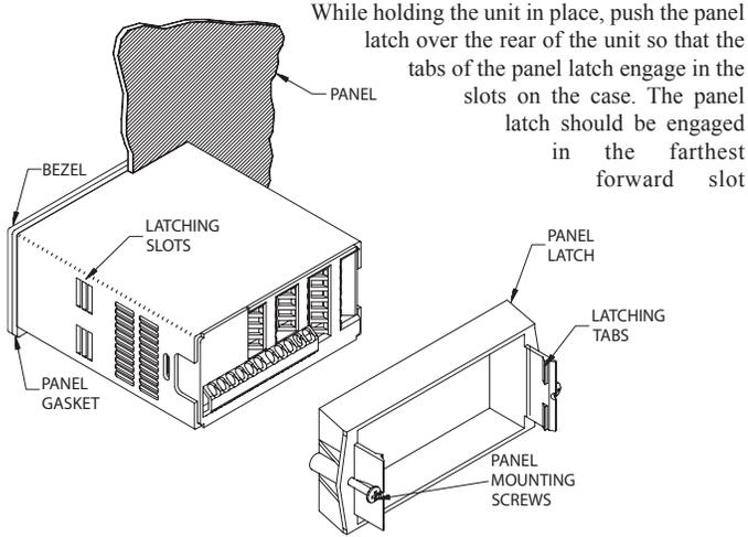
possible. To achieve a proper seal, tighten the latch screws evenly until the unit is snug in the panel (Torque to approximately 7 in-lbs [79N-cm]). Do not over-tighten the screws.
