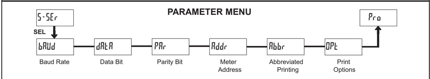
The Serial Setup Parameters are only active when one of the optional serial communications/programming cards is installed in the meter. Refer to the CUB5COM bulletin for details and setup for the CUB5 RS232 or RS485 serial communications. Refer to the CUB5USB bulletin for details on the CUB5 USB programming and programming requirements.
