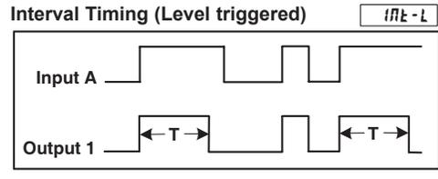
The input signal must be wired to both the Input A and User Input 1 terminals. The Timer Input plug jumper and the User Input plug jumper must both be set to the same position (either both SNK or both SRC).
