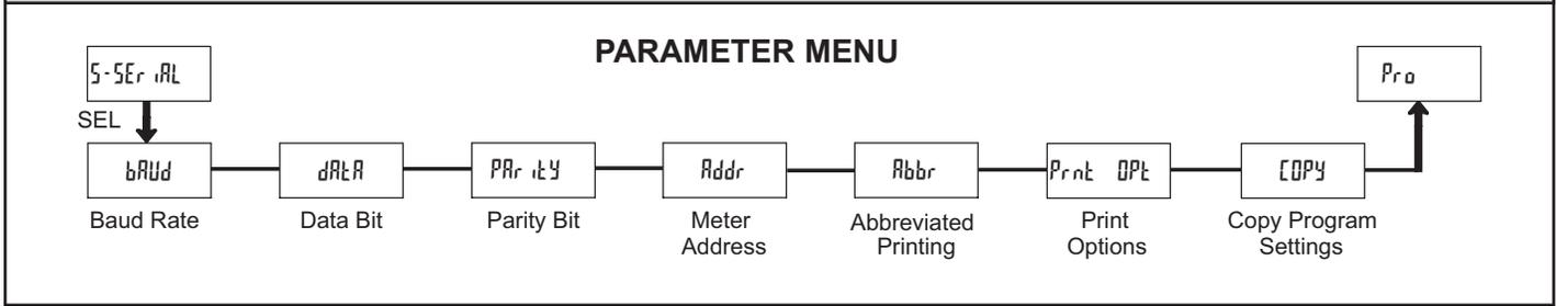
Module 5 is the programming module for the Serial Communications Parameters. These parameters are used to match the serial settings of the CUB5T with those of the host computer or other serial device. The Serial Setup Parameters are only accessible when an optional RS232 or RS485 serial communications module is installed in the meter.
