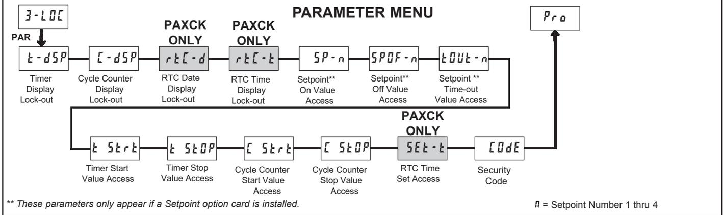
Module 3 is the programming module for setting the Display Lock-out Parameters and the "Quick Programming Mode" Value Access Parameters. In the Quick Programming mode, after the PROGRAM LOCKOUT PARAMETERS and before the Security Code (CODE), a Display Intensity Level (d-LEU) parameter is available when the security code is non-zero. It allows the display intensity to be set to 1 of 16 levels (0-15).
