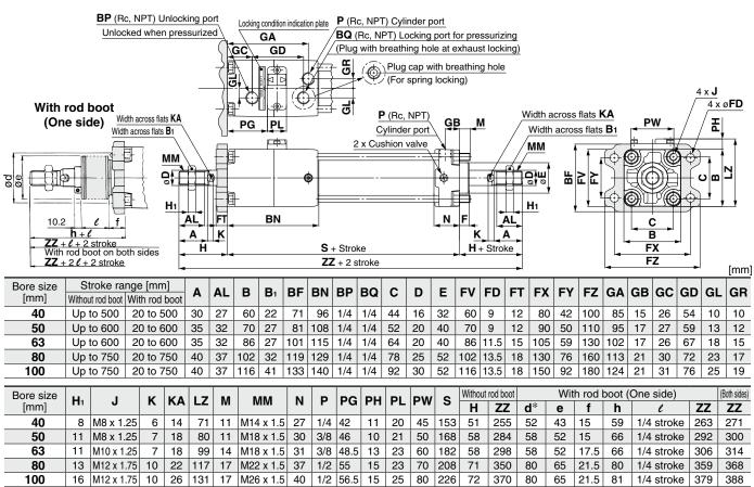
\* When a hole must be made to accommodate the rod portion, make sure to machine a hole that is larger than the outer diameter of the boot mounting bracket ød.
