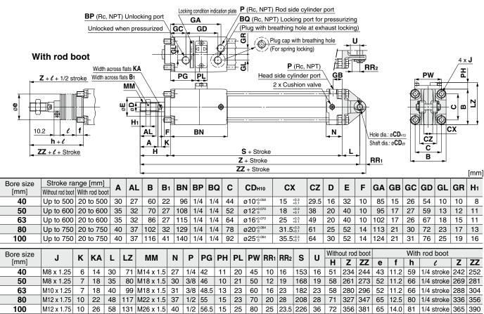
\* A clevis pin, flat washers and split pins are included.
