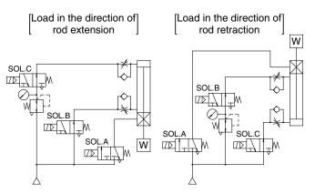
Note) The basic circuit examples are for spring locking (exhaust locking). For pneumatic locking (pressure locking) or spring and pneumatic locking, a 5 port solenoid valve should be installed in SOL.A.
