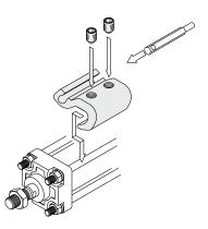
The figure shows the mounting example for the D-A9Ü(V)/M9U(V)/M9UW(V)/M9UA(V) types.
