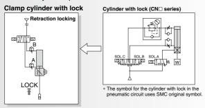
Able to maintain an unlocked state Assembly and maintenance simplified
