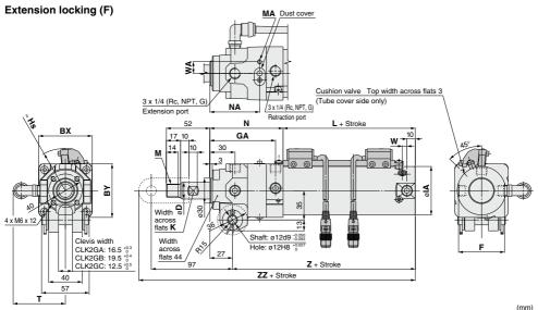
Symbol GA NA вх BY D F IΑ Κ L М MA N т w WA z ΖZ Hs Bore size 56 54 16 44 77 47 14 55 M12 x 1.5 M4 x 7 59 57 5 12.5 114 226 45.5 M16 x 1.5 M4 x 7 50 64 64 20 55 78.5 58 17 58 87.5 59.5 60 5.5 14 118.5 230.5 51 M16 x 1.5 M5 x 7 72 17 61 67 5.5 19 122 234 58.5
