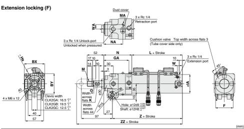
Symbol вх BY D GΑ IΑ κ L М MA NA т w WA z ΖZ Hs Rore size 40 56 54 16 44 77 47 14 55 M12 x 1.5 M4 x 7 86 59 57 5 12.5 114 226 45.5 50 64 64 20 55 78.5 58 17 58 M16 x 1.5 M4 x 7 87.5 59.5 60 5.5 14 118.5 230.5 51 63 74 74 20 69 82 72 58 M16 x 1.5 M5 x 7 61 67 5.5 19 122 234 58.5
