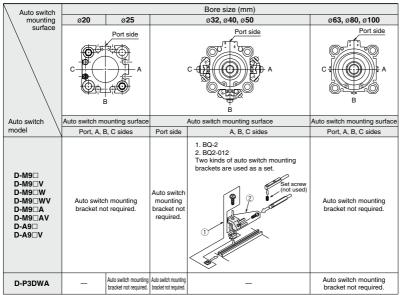
Note 1) For each cylinder series, when a compact auto switch is mounted on the three sides (A, B and C above) other than the port side of bore sizes ø32 to ø50, the auto switch mounting brackets above are required. Order them separately from cylinders.
