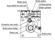
Locked condition (when air is exhausted.)
