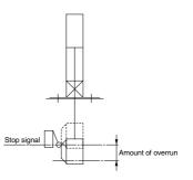
3. In order to further improve stopping accuracy, the time from the stop signal to the operation of the lock should be shortened as much as possible.
