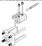
The above figure shows the mounting example of D-A9□(V)/M9□(V)/M9□W(V)/
