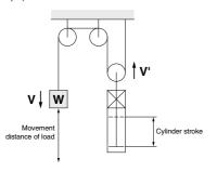
3. Shown below is an example of a model selection procedure for an intermediate stop application (including an emergency stop in operation). Only when locking in a drop prevention application, when no kinetic energy is applied, the maximum load mass should be determined by using graphs 5 through 7 on page 981 (taking into consideration the upper limit of the load mass at a maximum speed of 100 mm/s).
