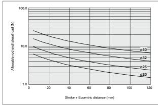
Allowable rod end lateral load can be found from the above graph. Do not apply a load beyond the line on the graph.
