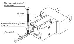
Note) Use a watchmaker's screwdriver with a grip diameter of 5 to 6 mm to tighten the auto switch mounting screw. The tightening torque should be about 0.05 to 0.15 N·m.
