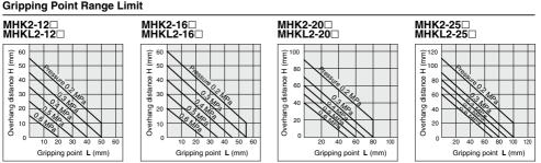
Note) Distance to the gripping point L of single acting type is shortened by spring return. Use air gripper within gripping force line shown for each pressure in effective gripping force graph
