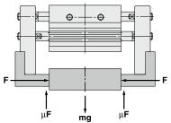
"Gripping force at least 10 to 20 times the workpiece weight"
