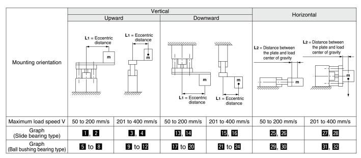
When the maximum speed exceeds 200 mm/s, the allowable load mass is determined by multiplying the value shown in the graph at 400 mm/s by the coefficient listed in the table below.
