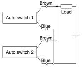
(Solid state) When two auto switches are connected in parallel, malfunction may occur because the load voltage will increase when in the OFF state.
