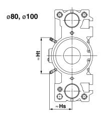
D-P4DW (\* Cannot be mounted on bore size ø25 or less)
