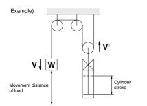
3. The following selection example and procedures are based on use at the intermediate stop (including emergency stops during operation). However, when the cylinder is in a locked state, kinetic energy does not act upon it. Under these conditions, use the load mass at the maximum speed (V) of 100 mm/s shown in graphs (5) to (7) on page 889 depending on the operating pressure and select models.
