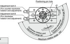
Note) • The drawing shows the rotation range of the positioning pin hole.
