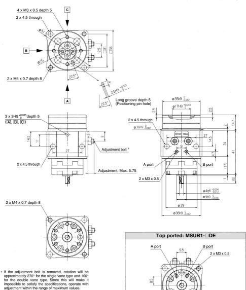
These drawings indicate the condition when the B port is pressurized.
