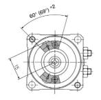
\* If the adjustment bolt is removed, rotation will be approximately 270° for the single vane type and 100° for the double vane type. Since this will make it impossible to satisfy the specifications, operate with adjustment within the range of maximum values.
