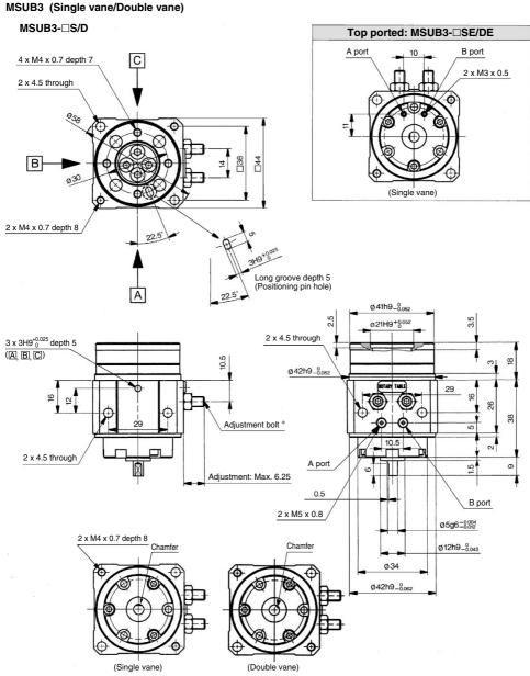
The outside drawings show the single vane type, but only the position of the chamfered sections shown in the above drawings differs from single and double vane.
