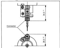
\* If the adjustment bolt is removed, rotation will be in the adjustment bott is removed, rotation will be approximately 270° for the single vane type and 100° for the double vane type. Since this will make it impossible to satisfy the specifications, operate with adjustment within the range of maximum values.
