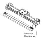
\* Stud fastening: After a temporary tightening, tighten an additional 1/4 turn.
