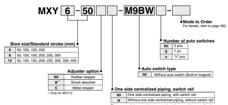
The auto switch cannot be mounted on the one side centralized piping type without switch rail (N).
