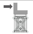
(2) The transferred object should be stopped in line with the center of the guide. If there is an offset in the  $L_2$  direction, an eccentric load will be applied to the guide. In this case, this product should not be used as a stopper.
