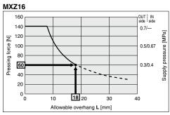
Allowable supply pressure on OUT side and IN side is the theoretical output of cylinder when pressing force is required.
