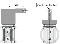
(3) Place a bracket so that it contacts the machined corner of the surface for mounting or insert a pin into the through hole on the side to prevent sliding.
