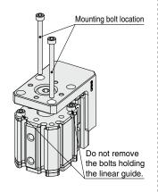
7. When mounting the product and a jig, tighten it with screws of appropriate length at an appropriate torque.
