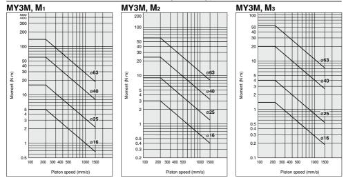
Select the load from within the range of limits shown in the graphs. Note that the maximum allowable moment value may sometimes be Maximum Allowable Load exceeded even within the operating limits shown in the graphs. Therefore, also check the allowable moment for the selected conditions.
