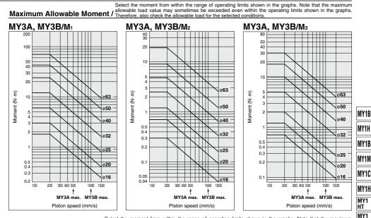
Select the moment from within the range of operating limits shown in the graphs. Note that the maximum allowable load value may sometimes be exceeded even within the operating limits shown in the graphs. Therefore, also check the allowable load for the selected conditions.
