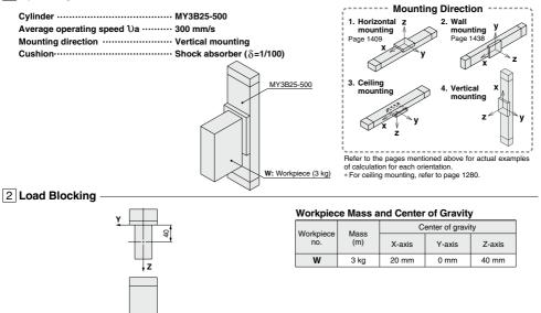
3 Calculation of Load Factor for Static Load -
