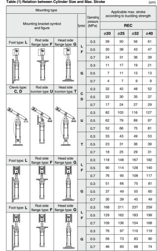
2) In the case where cylinder is used for dynamic action: Load factor  $\eta$  = 0.5 or less 3) In the case where guide is used in horizontal orientation: Load factor  $\eta$  = 0.9 or less
