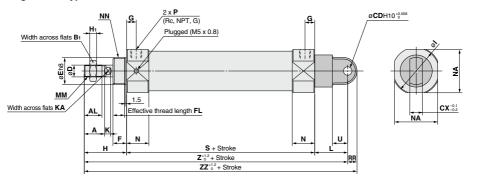
(mm) Bore (mm) Α ΑL В1 CD СХ D Ε F FL G н Нı 1 Κ KA L ММ N 20\_0,033 20 18 15.5 13 9 10 8 13 10.5 10 41 5 33.5 5 6 30 M8 x 1.25 20 22 19.5 17 10 10 26\_0.033 13 10.5 10 45 37.5 5.5 8 30 M10 x 1.25 20 25 9 6 32 22 19.5 17 9 10 12 13 10.5 11 45 6 46.5 5.5 10 30 M10 x 1.25 22 40 24 21 22 10 15 14 16 13.5 50 56.2 12 39 M14 x 1.5 26.5
