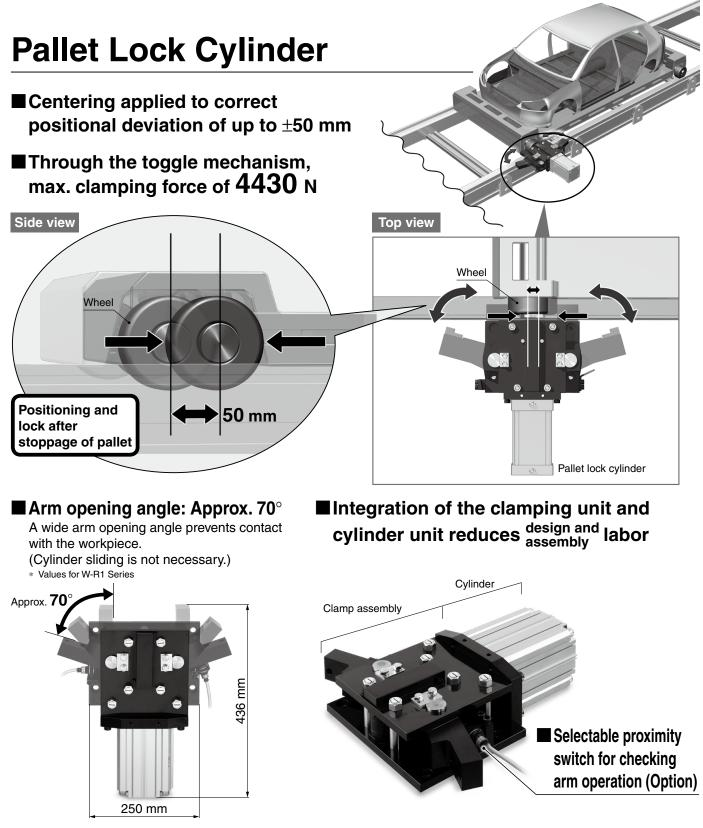
Selectable when the mass of the transferred object is either 1000 kg or 3000 kg, with consideration given to the impact during positioning
