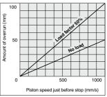
Condition/Driving pressure: 0.5 MPa Brake releasing pressure: 0.3 MPa Mounting orientayion: Horizontal
