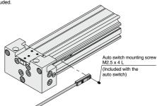
Note) When tightening an auto switch mounting screw, use a watchmaker's screwdriver with a handle of approximately 5 to 6 mm in diameter.
