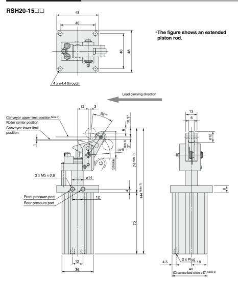
Note 1) The figure shows dimensions at the maximum energy absorption capacity.
