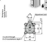
Bore size: Ø40, Ø50 RSQB50 -- DBZ (Double acting) ransfer direction 13.5\*5 31 Width across 10 7.5 2 x (Rc, NPT, G) 1/8 flats K a20 Adjustment bolt 24.5 Ę 28 4 x ø**N** through B + Stroke 100 + Stroke
