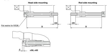
Note) Use the attached washer when inserting the bolt from the rod side.
