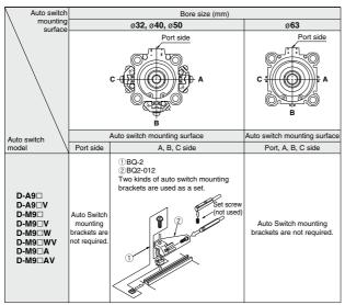
Note 1) When a compact auto switch is mounted on the three sides (A, B and C above) other than the port side of bore sizes ø32 to ø50, the auto switch mounting brackets above are required. Order them separately from cylinders.
