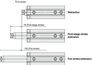
\* Consult with SMC for the special tube for intermediate strokes of a full stroke.
