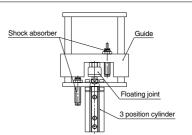
6. When the kinetic energy of a load (non-moving parts and moving parts) exceeds the allowable kinetic energy in table 3, it also exceeds the cushioning capacity of the rubber bumper. Add a cushioning mechanism such as a shock absorber shown in the figure above.
