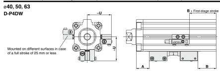
Auto Switch Proper Mounting Position \* The values in the table below should be used as a reference for the auto switch mounting position at the stroke end detection. Adjust the auto switch after confirming the operating conditions in the actual setting.
