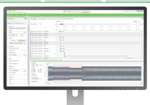
Designed to provide advanced diagnostic information to EcoStruxure Power software for power quality analysis and system forensics. Graphical event analysis makes it easy to see what happened and provides the contextual information needed to quickly draw conclusions about cause and effect.
