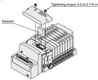
Remove the cover from the side of the end plate and remove the old element with a flat blade screwdriver, etc.
