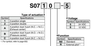
\*1: Not compatible with dual 3-port valves. Base mounted plug-in
