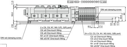
L2 = L1 - 10.5  $L3 = 8.5 \times n1 + 46$   $L4 = L3 + 97.5 + 47 \times n2$  L5 = (L1 - L4)/2  $L6 = 8.5 \times n1 + 31$  $L7 = 47 \times n2 + 86.1$
