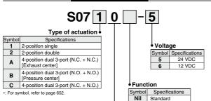
External pilot\*1 Base mounted plug-in \*1: Not compatible with dual 3-port valves.
