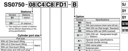
\*1: When installing a back pressure check valve on the required station, enter the part number and specify the station position on the manifold specification
