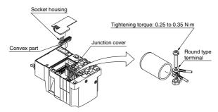
4 Take out the socket housing and connect the black and white lead wires. The connection layout is common to all kits.
