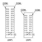
Mixed single and double wiring are available as an option. The maximum number of manifold stations is determined by the number of solenoids. Count one point for a single solenoid type and two points for a double solenoid type. The total number of solenoids (points) must not exceed 24 for 26P, 18 for 26P.
