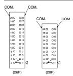
Mixed single and double wiring are available as an option. The maximum number of manifold stations is determined by the number of solenoids. Count one point for a single solenoid type and two points for a double solenoid type. The total number of solenoids (points) must not exceed 24 for 26Pt. 18 for 20Pt.
