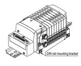
It is used for mounting a manifold on a DIN rail. The DIN rail mounted bracket is fixed to the manifold end plate. (The specification is the same as that for the option -D.) 1 set of DIN rail mounting bracket is included for 1 manifold (2 or 3 DIN rail mounting brackets (S. T kit)).
