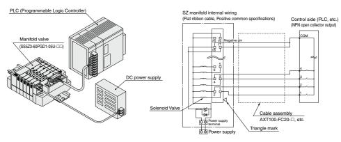
Wiring example when not using manifold power supply terminal (Power is supplied to the control side or along the wiring, etc.)
