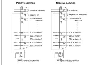
• The maximum number of stations that can be accommodated is 20 manifold stations, with up to 21 solenoids.
