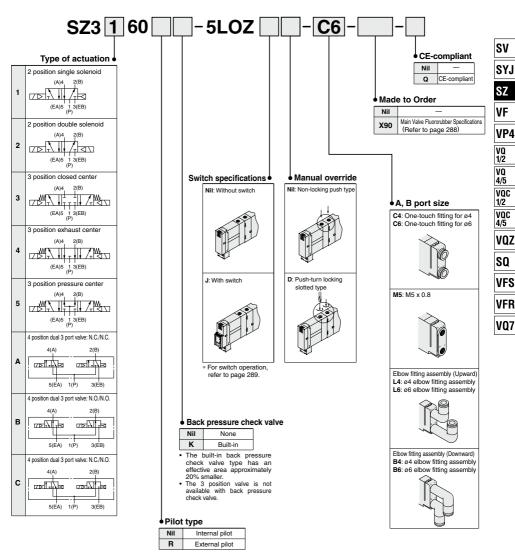
Dual 3 port valves are not available with external pilot specifications.
