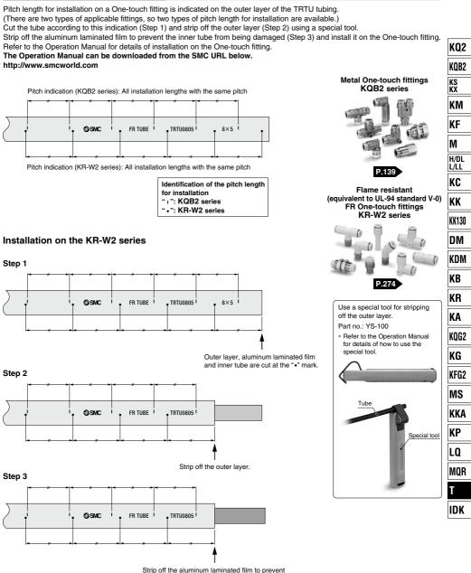
Strip off the aluminum laminated film to preven the inner tube from being damaged.
