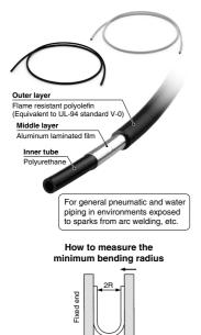
Bend the tube into the U-form at a temperature of 20°C. Fix one end and close loop gradually. Measure 2R when the deformed ratio of the tube diameter at bending reaches 5%.
