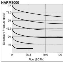
Pressure Characteristics Supply pressure 100 psig Secondary pressure 30 psig Flow rate .7 SCFM
