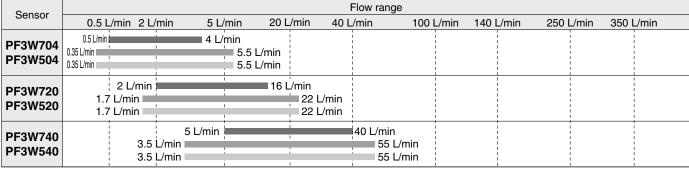
\* For the PF3W5 series, the display flow range and set flow range are the same as those of the flow monitor PF3W3 series. Rated flow range Display flow range Set flow range
