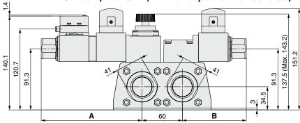
Supply unit Unit components: S (With flow adjustment valve)
