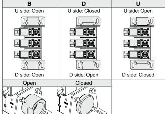
When "Open," the port size of the main piping is 1 inch.
