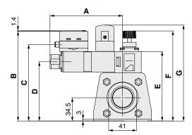
Flow switch: Remote sensor unit (With temperature sensor) Unit components: None
