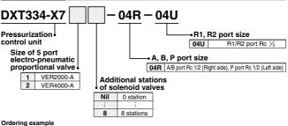
DXT334-X711-04R-04U------ 1 pc VS7-8-FG-D-3M ..... ···· 1 pc. (Third station of manifold where 1 piece of "VS7-8-FG-D-3M" is added to the basic unit of "VER2000-A" and "VS7-8-FG-S-3N".)
