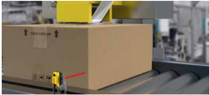
Single-Point Leading Edge Detection
