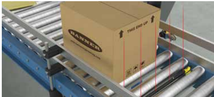
Through the Roller Leading Edge Detection
