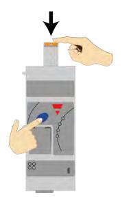
Fig. 1 Hold the blue button while powering up the NRGC-PN
