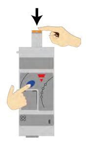
Fig. 1 Hold the blue button while powering up the NRGC-EIP
