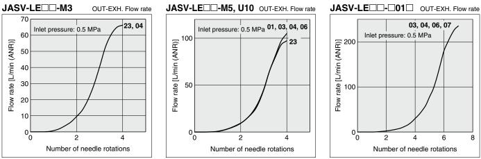
\* The numbers above the flow rate characteristic curves in the charts show the applicable tubing outside diameter as defined by the product number.
