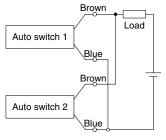
(Solid state) When two auto switches are connected in parallel, malfunction may occur because the load voltage will increase
