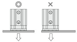
• If multiple magnet grippers are used for transferring a workpiece with a large surface area, properly allocate the magnet grippers to maintain balance.
