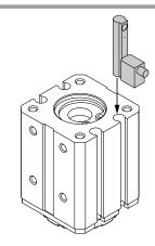
2. Keep a gap wider than the values listed in the table when arranging the magnet grippers side by side or when placing the magnet grippers close to magnetic objects such as iron.
