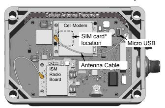
Figure 5. Internal view of a DXM1200
