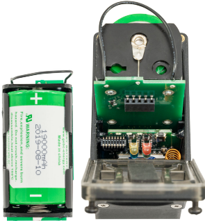
Figure 1. Battery pack and board
