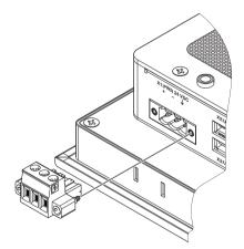
Connect a power source to the three-position removable connector. The connector (Order No. 1777992) accepts wire sizes from 0.2 to 2.5 mm<sup>2</sup> (24 to 12 AWG). Torque the wire-retaining screws in the connector to 0.5 Nm (4.4 lb<sub>f</sub>-in.).
