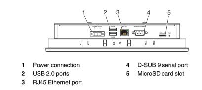
Figure 3-4 Connectors and ports
