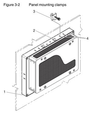
2. From the front, place the bottom edge of the WP 6...PS in the opening (1), making sure the spring-loaded retention clips (2) are inside the panel. Tilt the top of the WP 6...PS into the opening until the retention clips are inside the panel. Ensure that the gasket is properly positioned in the groove and against the panel.
