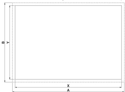
1. Cut a hole in the enclosure according to the dimensions for the selected display.
