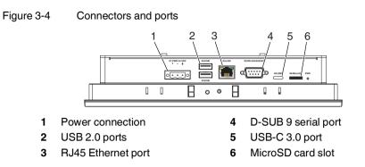
After mounting the WP 6...PS, make any necessary cable connections. The available connectors are:
