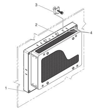
Figure 3-2 Panel mounting clamps
