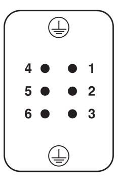
Connector pin assignment, connection side
