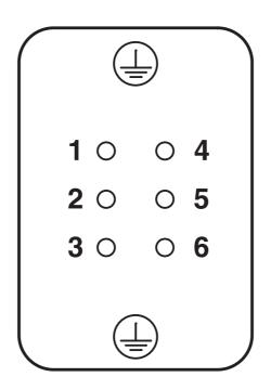
Connector pin assignment, connection side
