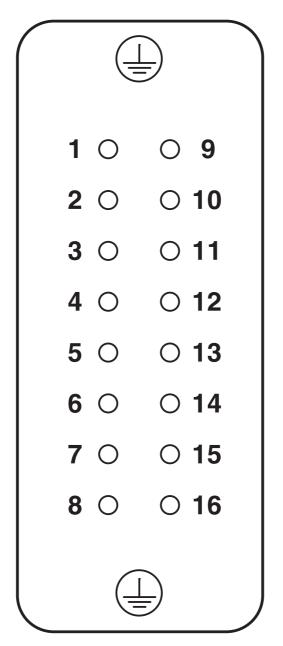
Connector pin assignment, connection side
