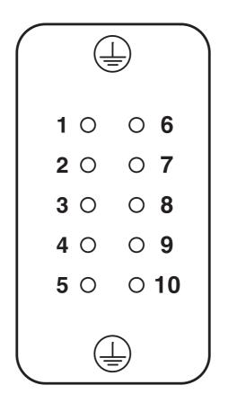
Connector pin assignment, connection side
