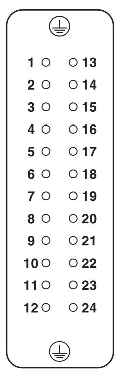
Connector pin assignment, connection side
