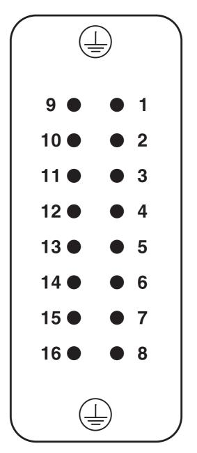
Connector pin assignment, connection side
