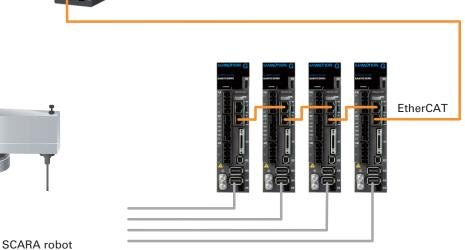
Automatic coating machine (Model no. SMC100-A) Interpolation control, etc.
