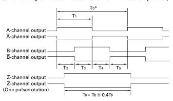
$^{\ast}\,T_{0}$  is the average time for one encoder rotation when the encoder is rotated at a constant speed.
