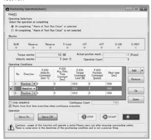
Servo motor test runs can be performed easily by issuing velocity commands and position commands from a PC. (Shows position jog operation)
