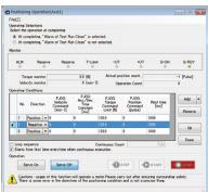
Servo motor test runs can be performed easily by issuing velocity commands and position commands from a PC. (A position jog screen is shown)
