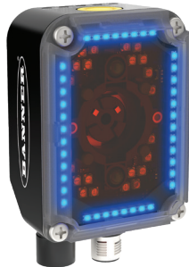
Multicolored LEDs for bright-field and dark-field illumination
