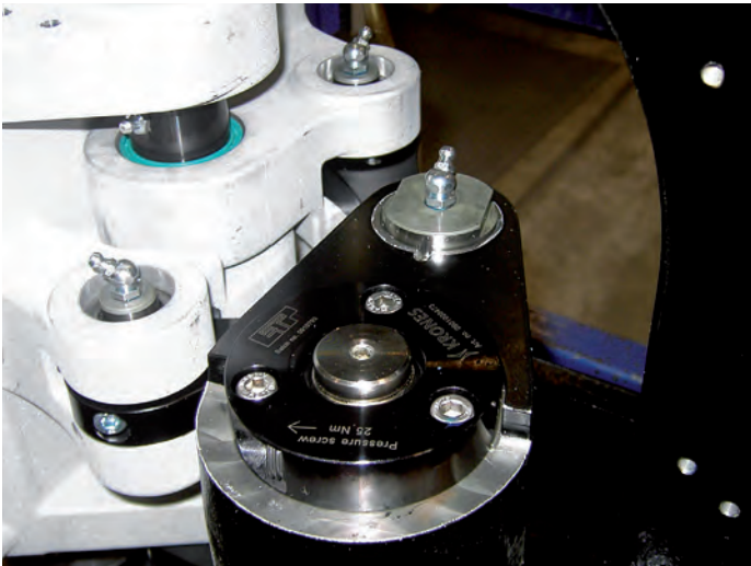
Lever fastened with ETP-EXPRESS to open/close the mold.
