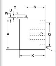
**NOTE:** The Actuating Pin Assembly is a simple pin which is forced out radially from the main body when overload occurs. When using this option, it is important to note that the housing (F bore) or external mounting hub end of the unit is the power source or input end. This part of the unit must continue to rotate for the extended pin to contact a customer supplied limit switch for shutdown or warning.
