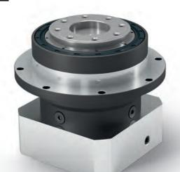
The **PFHE** represents an economically attractive alternative for high-load applications in which high radial loads occur. The combination of special pre-stressed inclined roller bearings and a flanged output shaft in accordance with ISO 9409-1 gives the **PFHE** a very high load capacity. Thanks to the radial shaft seal that is used, this gearbox achieves protection class IP65 at the output side and can therefore also withstand adverse usage conditions.
