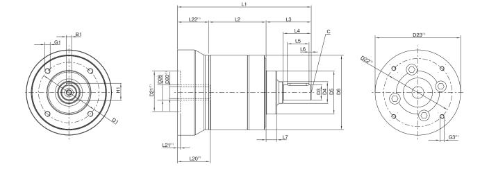
Drawing corresponds to a HLAE070 / 1-stage / output shaft with feather key / 11 mm clamping system / motor adaptation – one part / B5 flange type motor
