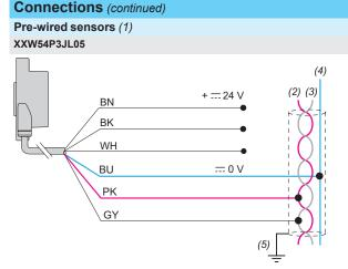
(1) Connecting the detector to the XXZBOX01 configuration interface with the XZCC12MDM40B connector: BN (Brown), WH (White), BU (Blue), BK (Black).
