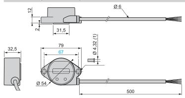
XXZKITDM6 cable with Deutsch DTM04 connector for sensor configuration
