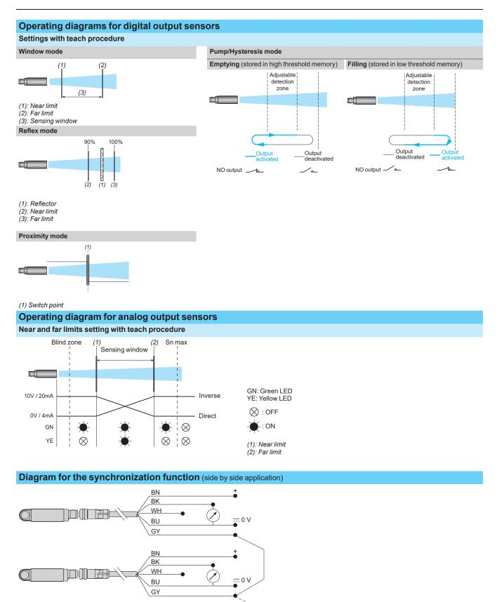
**NB**: To enable synchronization between several sensors, all of the wires of pin no.5 (gray) must be electrically connected together. A maximum of 8 sensors can be synchronized. To enable "Multiplexer" function for the sensors, use the XX Configuration Software. Without synchronization or multiplexing, the sensors must be at least 50 cm away from each other in order to avoid mutual interference.
