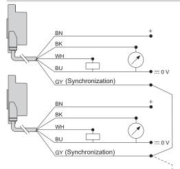
Note: Synchronization is recommended if more than one sensor is used in the same direction in order to avoid any interference between sensors due to the width of their beam. Up to 8 sensors can be synchronized to operate side by side by electrically connecting all pin no. 6 (gray) wires together. All sensors must be the same model and have the same cycle time setting.
