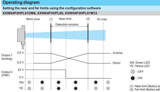
(1): Near limit (factory setting: 425 mm) (2): Far limit (factory setting: 3 m)
