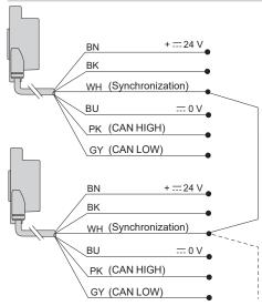
Note: Synchronization is recommended if more than one sensor is used in the same direction in order to avoid any interference between sensors due to the width of their beam. Up to 8 sensors can be synchronized to operate side by side by electrically connecting all pin no. 4 (white) wires together. All sensors must be the same model and have the same cycle time setting.
