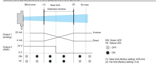
Note: The sensor's analog output emits 2 mA when it detects excessive environmental noise.
