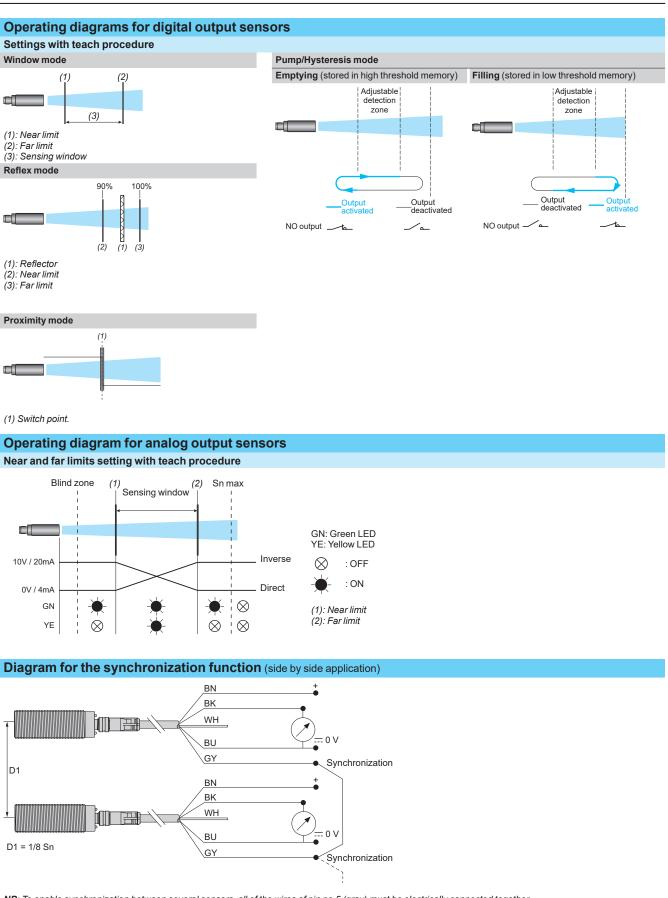
**NB**: To enable synchronization between several sensors, all of the wires of pin no.5 (gray) must be electrically connected together. A maximum of 8 sensors can be synchronized. To enable "Multiplexer" function for the sensors, use the XX Configuration Software. Without synchronization or multiplexing, the sensors must be at least 50 cm away from each other in order to avoid mutual interference.
