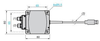
(1) Male M12 connector, 5-pin: power supply
