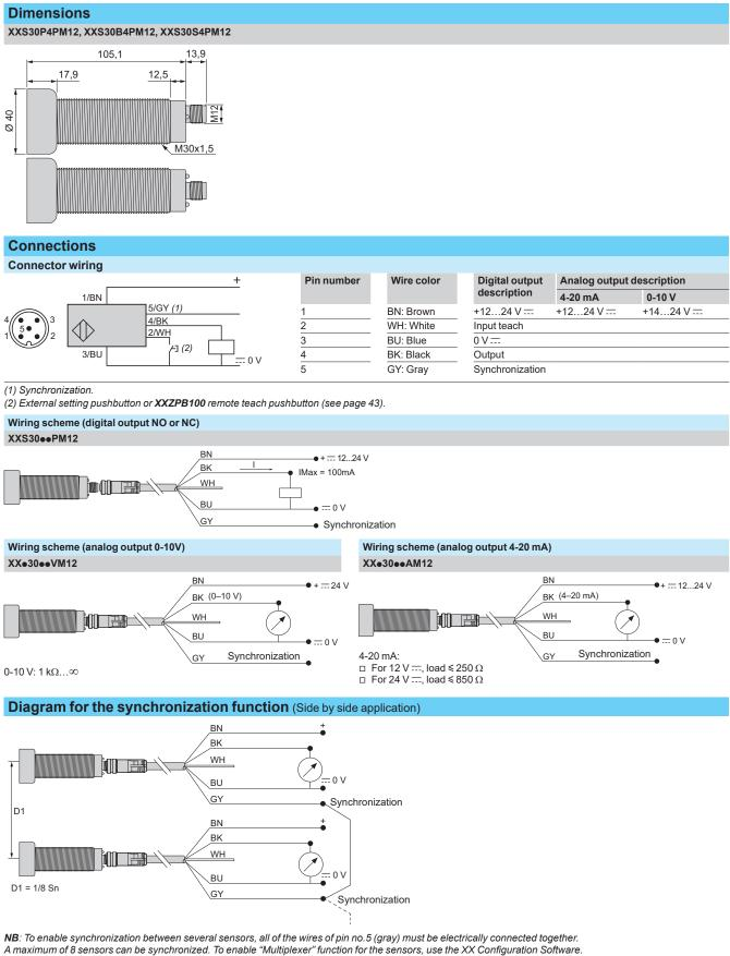
Without synchronization or multiplexing, the sensors must be at least 50 cm away from each other in order to avoid mutual interference.
