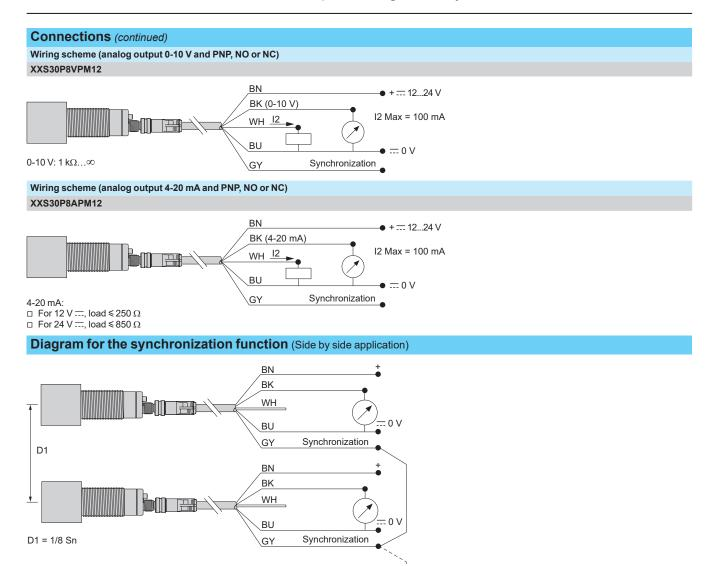
**NB**: To enable synchronization between several sensors, all of the wires of pin no.5 (gray) must be electrically connected together. A maximum of 8 sensors can be synchronized. To enable "Multiplexer" function for the sensors, use the XX Configuration Software. Without synchronization or multiplexing, the sensors must be at least 50 cm away from each other in order to avoid mutual interference.
