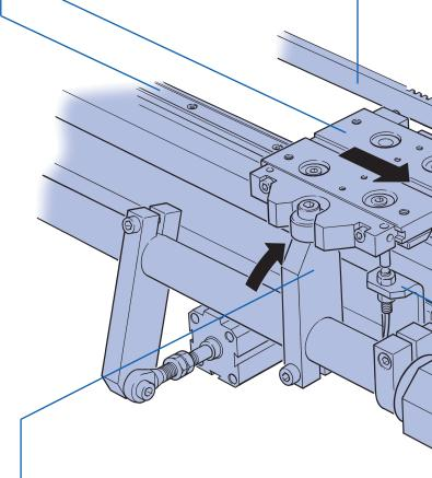
Carriage Locking System (optional with intermittent motion): Aligns specific carriages to a repeatable position anywhere along any straight section of the circuit to +/-0.05 mm.
