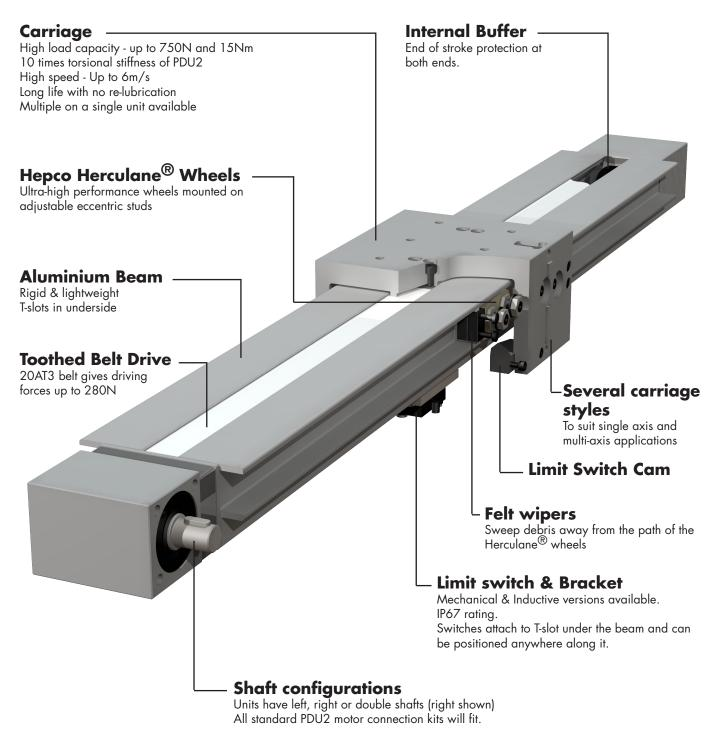
The unit shown has a right-handed shaft and a right-handed carriage
