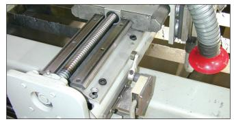
This multi-axis plasma cutter, using a LoPro ball screw driven system, operates in a harsh environment consisting of smoke, abrasive dust, weld splatter, hot sparks and elevated temperatures.
