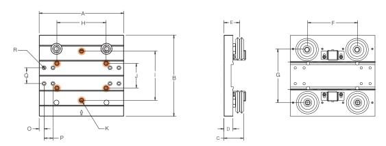
Above wheel plate assembly shown with track lubricators. Wheel plate assemblies are included with complete systems. See system ordering information, page 36.
