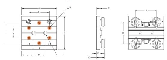
Above wheel plate assembly shown with track lubricators. Wheel plate assemblies are included with complete systems. See system ordering information, page 27.
