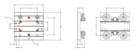
Above wheel plate assembly shown with track lubricators. Wheel plate assemblies are included with complete systems. See system ordering information, page 45.
