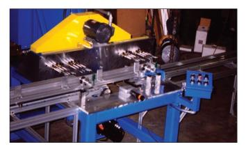
LoPro's precise travel and fast acceleration allow exact and repeatable hole drilling for door manufacturing, despite the presence of carbon fiber debris.
