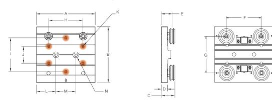
Above wheel plate assembly shown with track lubricators. Wheel plate assemblies are included with complete systems. See system ordering information, page 17.
