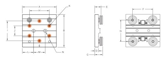
Above wheel plate assembly shown with track lubricators. Wheel plate assemblies are included with complete systems. See system ordering information, page 52.
